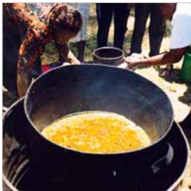
9.7 Molten combs heating with water in a water bath made from one metal container inside an oil drum half full of water, heated by fire underneath Tanzania © NB
