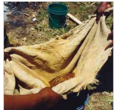
9.9 Filtering the molten beeswax and water mixture through hessian sacking Tanzania © NB
