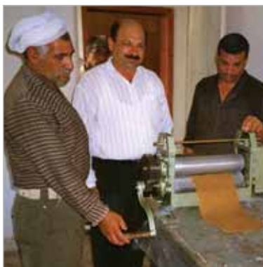
9.11 Using an embossed roller to make foundation in Iraq © NB
